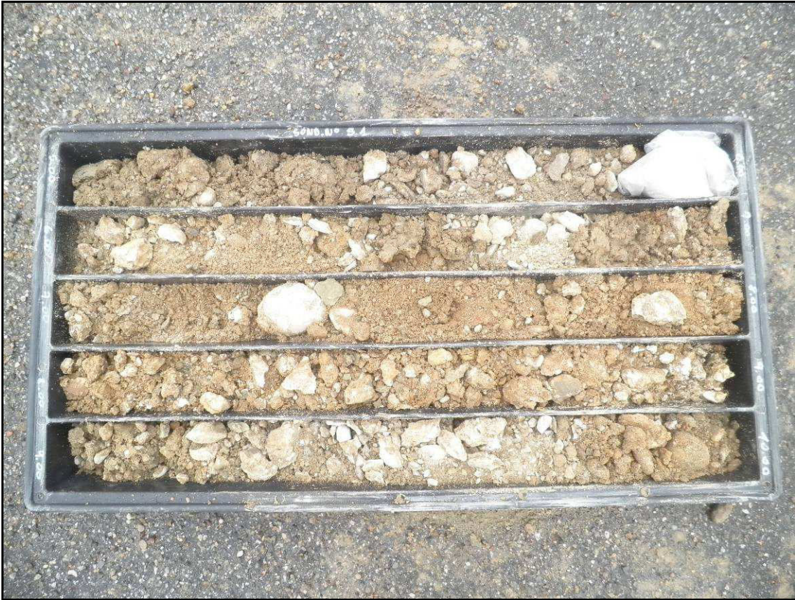
Sondaggio S1 da m 5,0 a 10,0 m.
