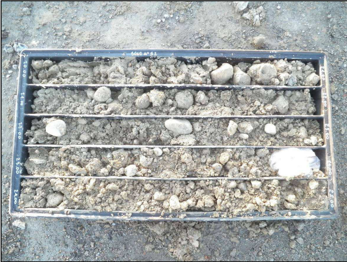
Sondaggio S2 da m 20,0 a 25,0 m.
