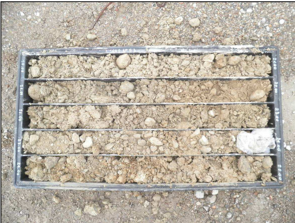
Sondaggio S3 da m 20,0 a 25,0 m.
