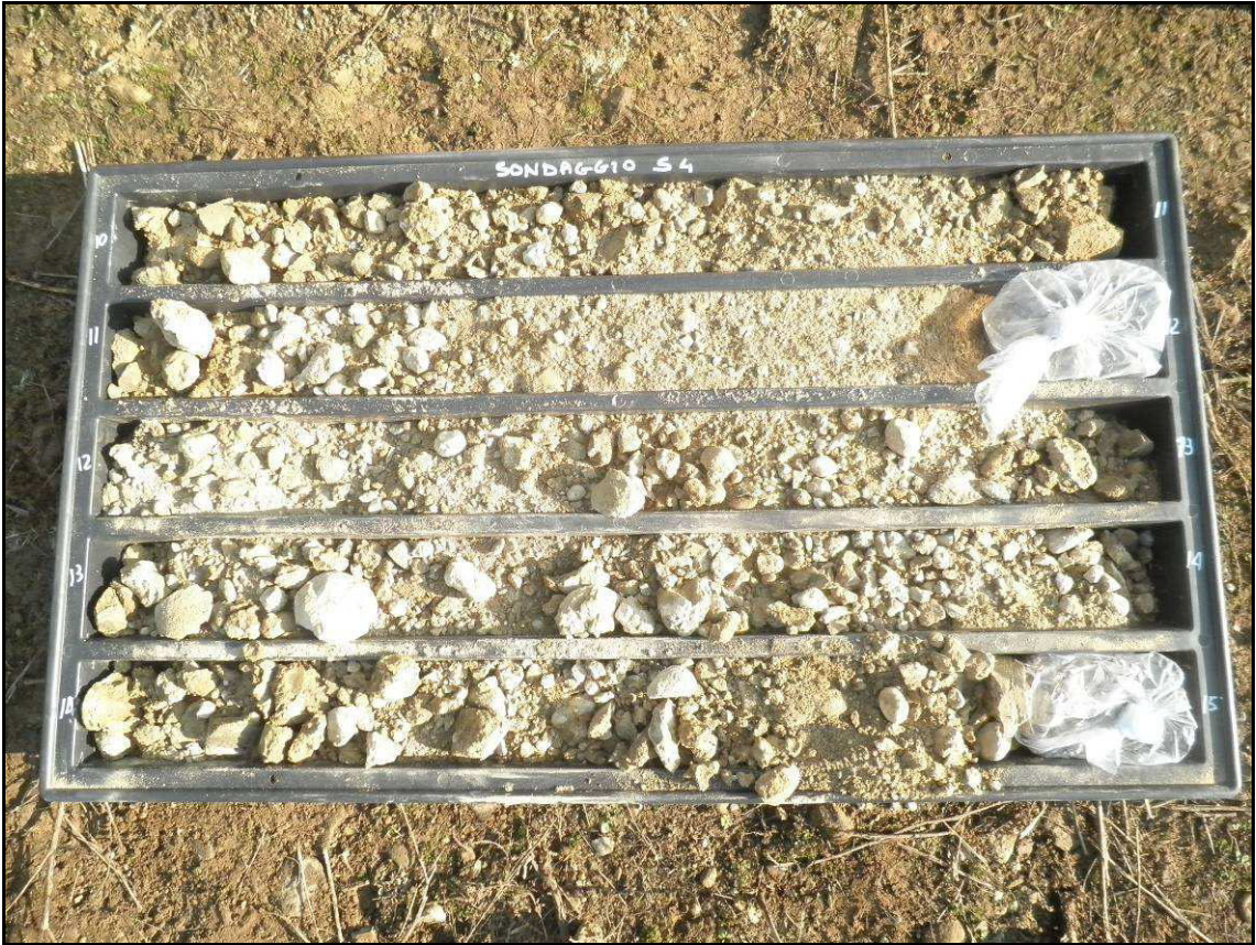
Sondaggio S4 da m 10,0 a 15,0 m.
