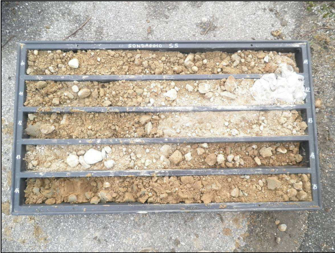
Sondaggio S5 da m 10,0 a 15,0 m.
