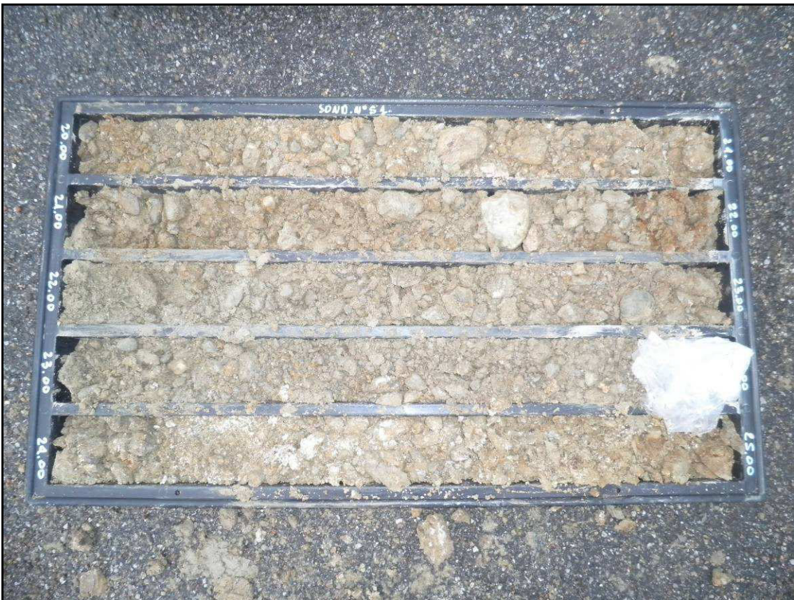
Sondaggio S1 da m 20,0 a 25,0 m.
