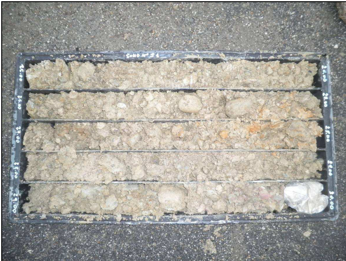
Sondaggio S1 da m 25,0 a 30,0 m.
