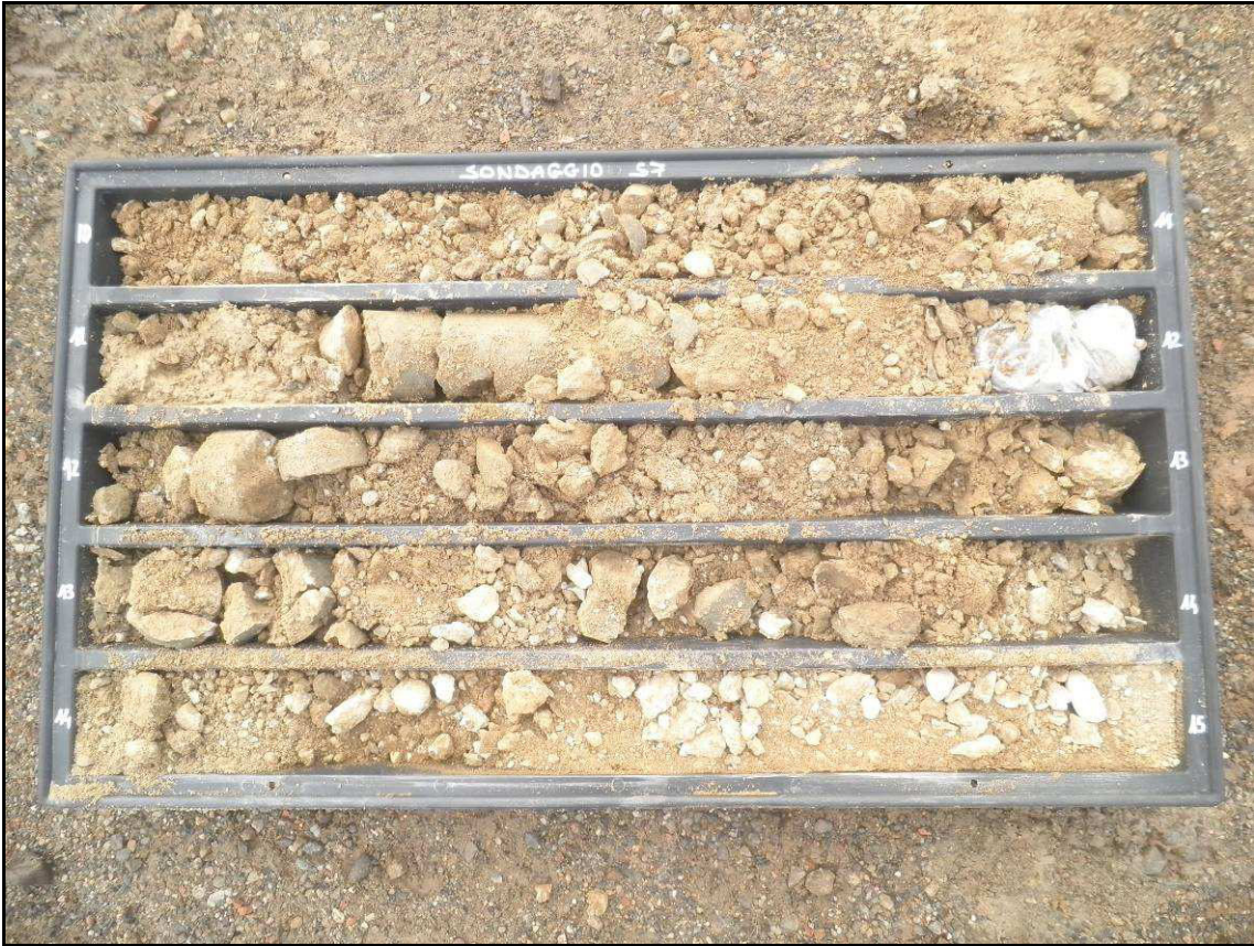
Sondaggio S7 da m 10,0 a 15,0 m.
